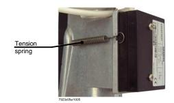
The AGA63.5A27 is to be secured to the SKPx5... or SKL25... by means of 2 tension springs. First, hook the open eye of the spring in the aluminium base between the black covers of the SKPx5... or SKL25... Then, hook the closed eye in the recess of the AGA63.5A27.
