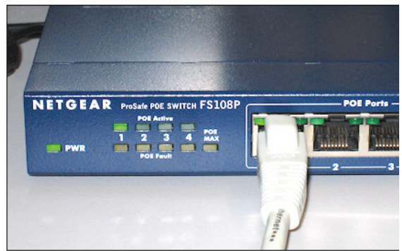
Example 2: Power over Ethernet Switch Compatibility: IEEE802.3af
